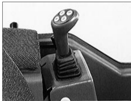
Automatic transmission is used with joystick steering.
